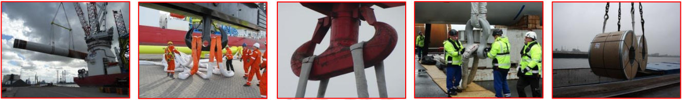
Example of stable fit round sling
